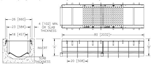
SPECIFYING ENGINEER IS RESPONSIBLE FOR CONCRETE ENCASEMENT AND REINFORCING BASED UPON APPLICATION AND LOCAL CODES
